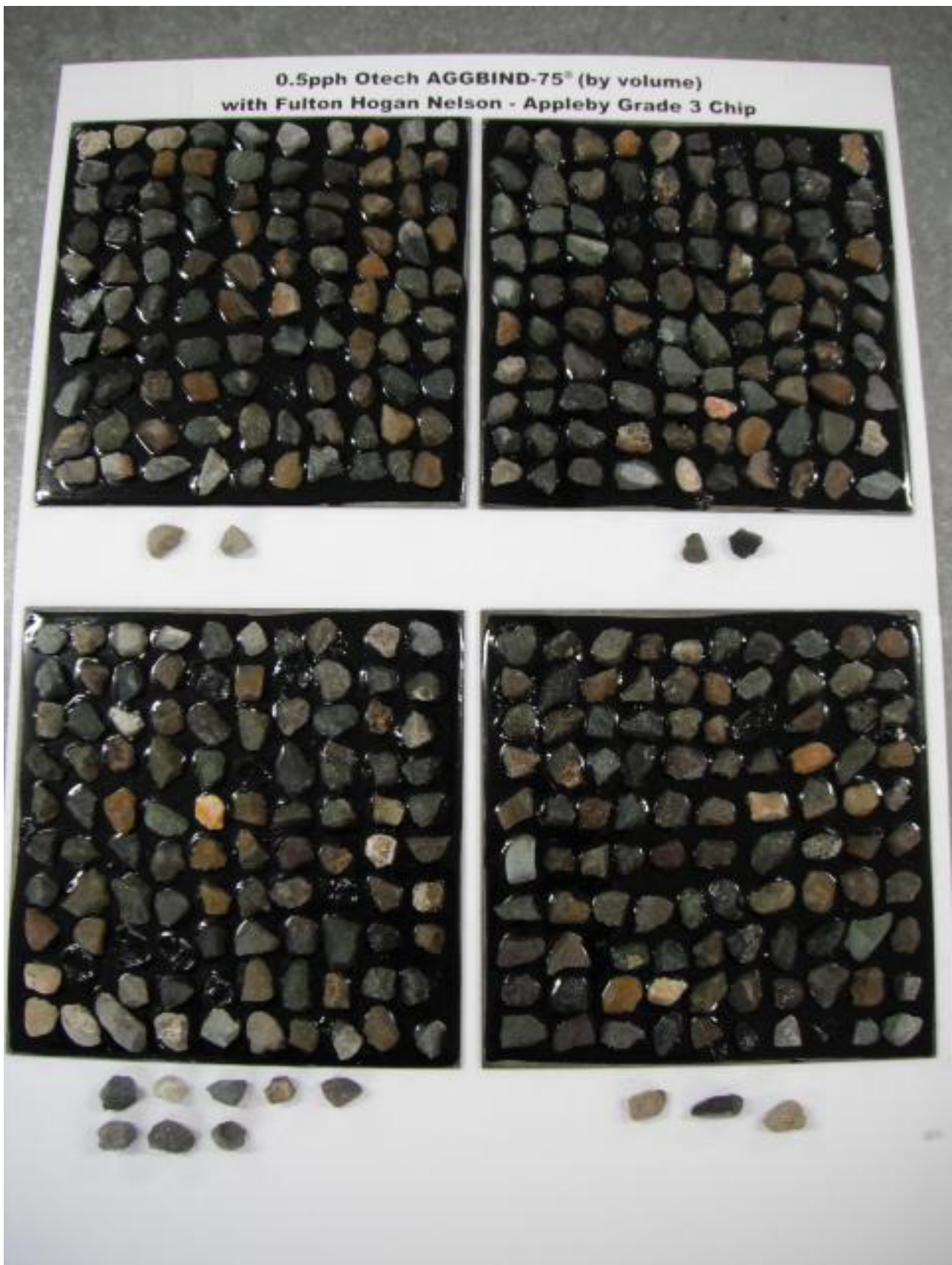
Figure 1. Photograph showing test plates with 180/200 bitumen and 0.7pph Otech AGGBIND-75® (by volume) after test was performed. Appleby grade 3 chip that was dislodged is arranged below the plates.
