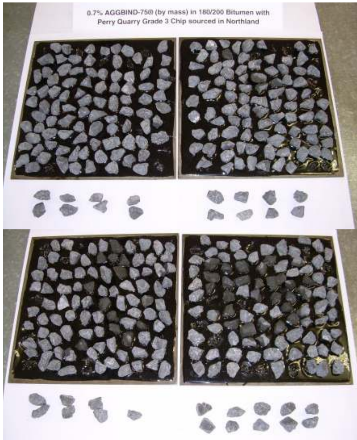
Figure 1. Photograph showing Vialit plates with 180/200 bitumen and 0.7% AGGBIND-75® (by mass) after test was performed. Grade 3 Perry Quarry chip that was dislodged is arranged below the plates.
