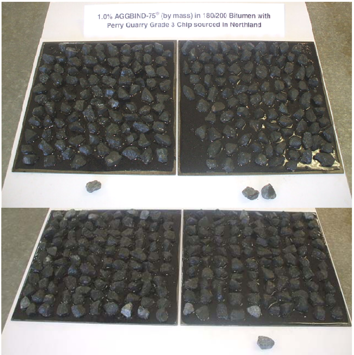
Figure 1. Photograph showing Vialit plates with 180/200 bitumen and 1.0% AGGBIND-75® (by mass) after test was performed. Grade 3 Perry Quarry chip that was dislodged is arranged below the plates.
