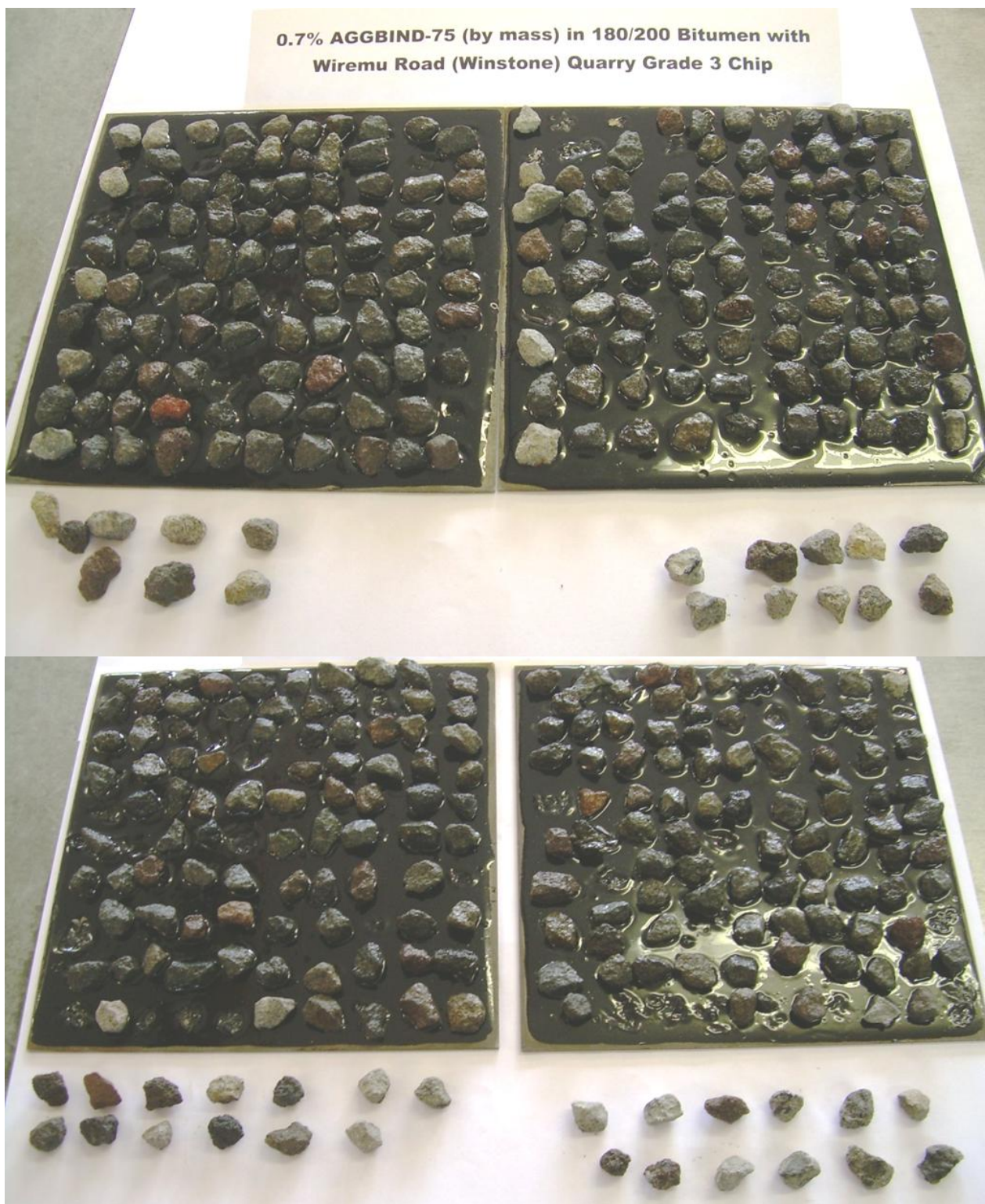
Figure 1. Photograph showing Vialit plates with 180/200 bitumen and 0.7% Otech AGGBIND-75 ® (by mass) after test was performed. Grade 3 Wiremu Road Quarry chip that was dislodged is arranged below the plates.
