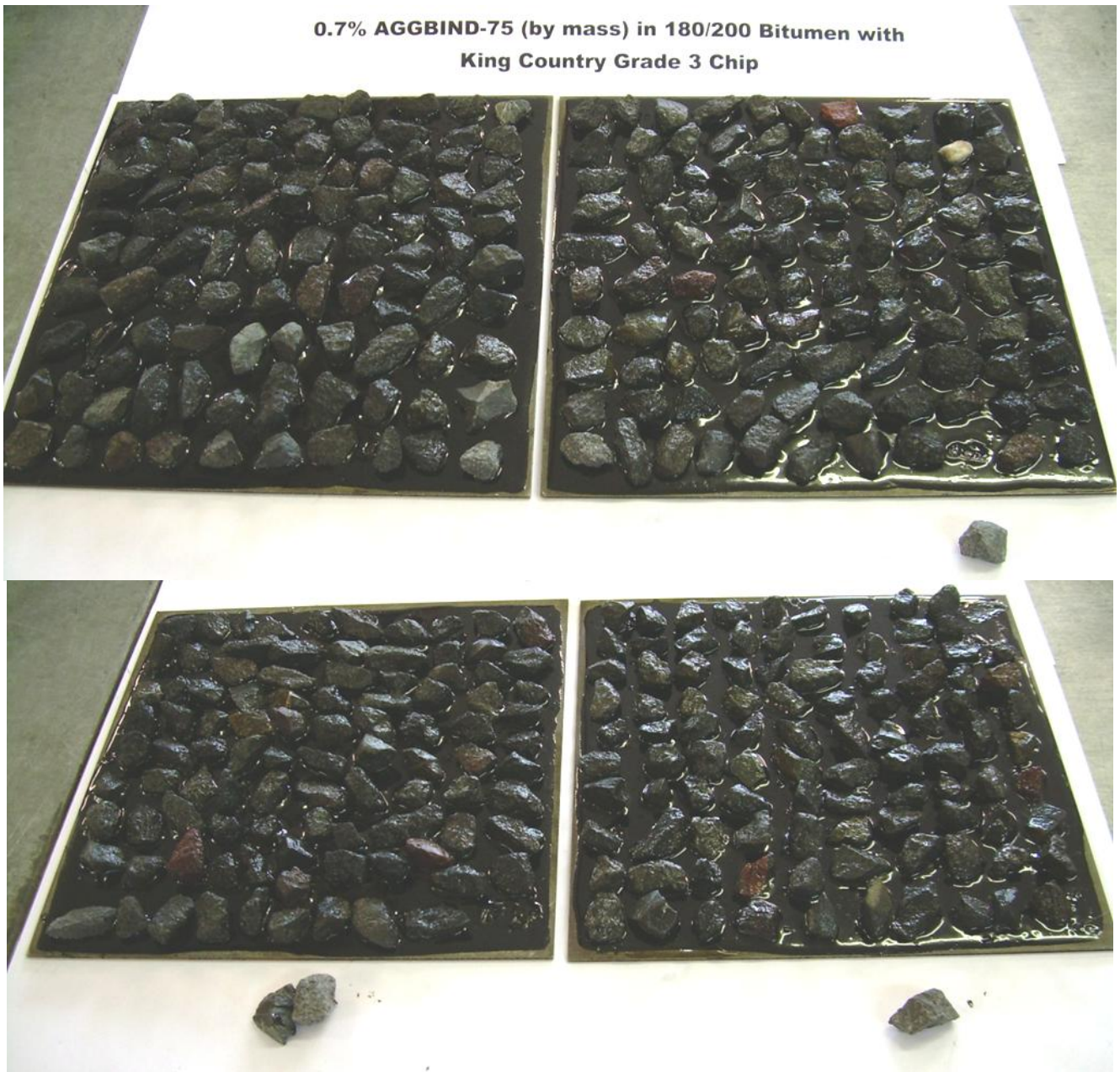
Figure 1. Photograph showing Vialit plates with 180/200 bitumen and 0.7% Otech AGGBIND-75® (by mass) after test was performed. Grade 3 King Country Quarry chip that was dislodged is arranged below the plates.
