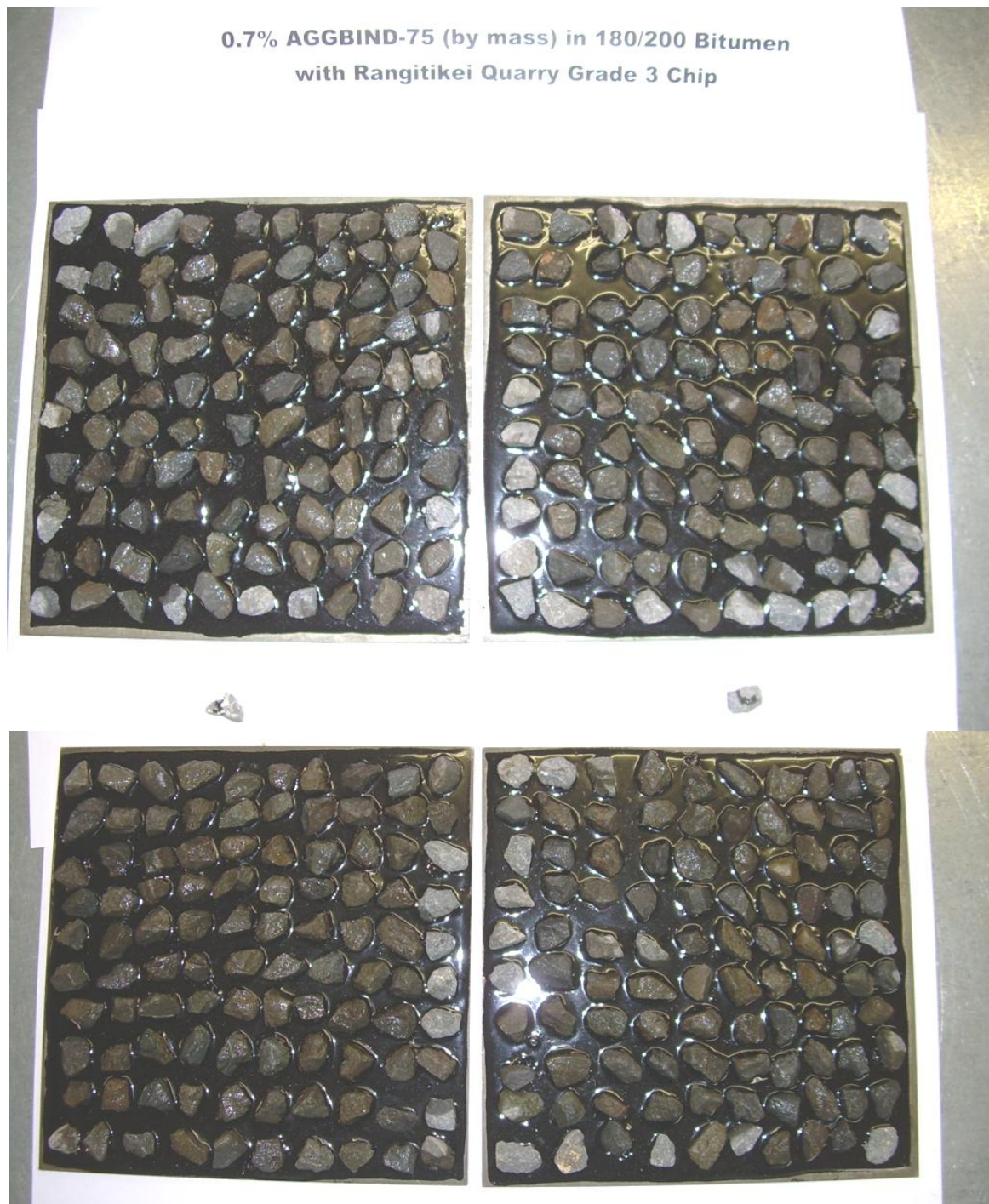
Figure 1. Photograph showing Vialit plates with 180/200 bitumen and 0.7% Otech AGGBIND-75 ® (by mass) after test was performed. Grade 3 Rangitikei chip that was dislodged is arranged below the plates.
