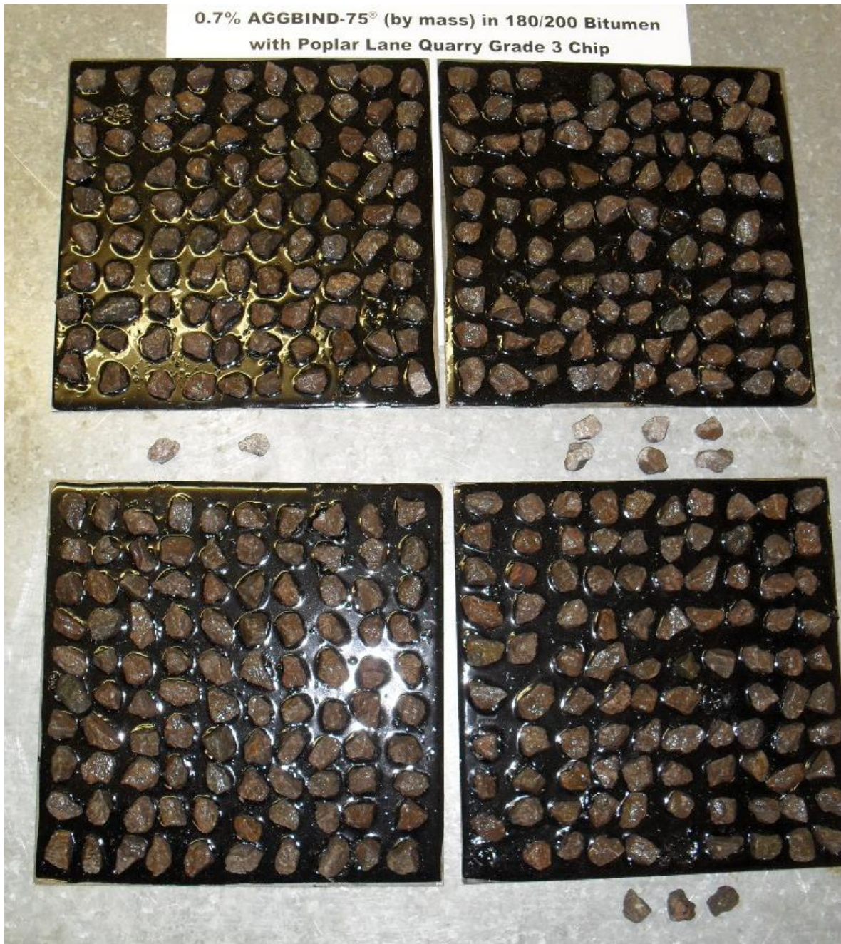
Figure 1. Photograph showing test plates with 180/200 bitumen and 0.7% Otech AGGBIND-75® (by mass) after test was performed. Poplar Lane Quarry grade 3 chip that was dislodged is arranged below the plates.
