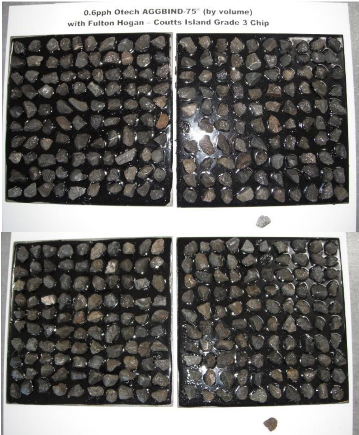
Figure 1. Photograph showing test plates with 180/200 bitumen and 0.6pph Otech AGGBIND-75® (by volume) after test was performed. Fulton Hogan – Coutts Island grade 3 chip that was dislodged is arranged below the plates.
