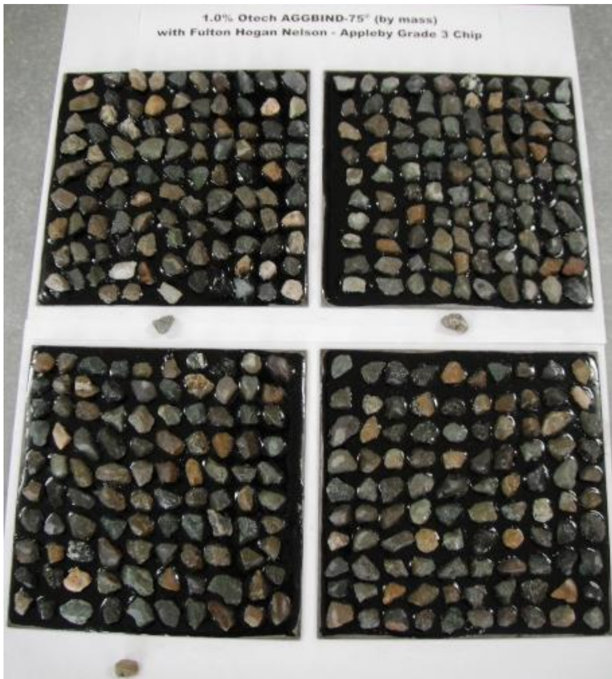
Figure 1. Photograph showing test plates with 180/200 bitumen and 1.0% Otech AGGBIND-75 ® (by mass) after test was performed. Appleby grade 3 chip that was dislodged is arranged below the plates.
