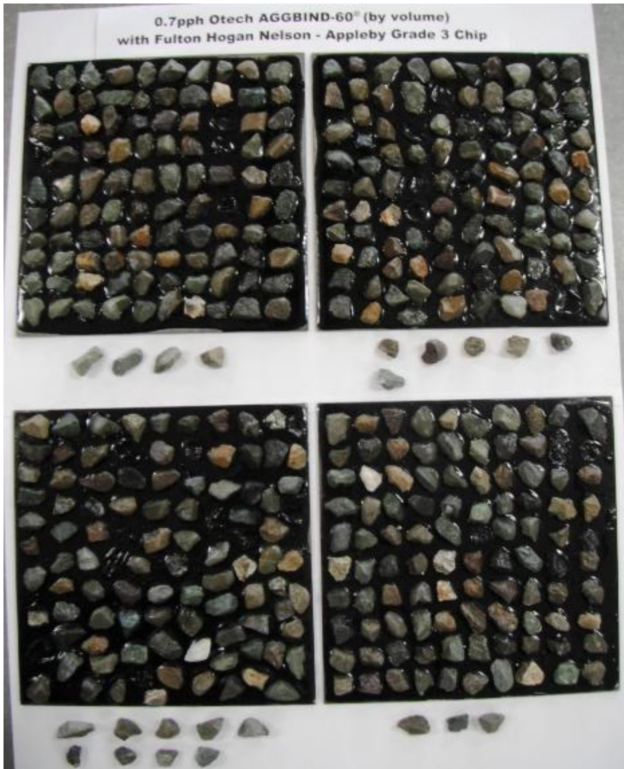
Figure 1. Photograph showing test plates with 180/200 bitumen and 0.7pph Otech AGGBIND-60® (by volume) after test was performed. Appleby grade 3 chip that was dislodged is arranged below the plates.
