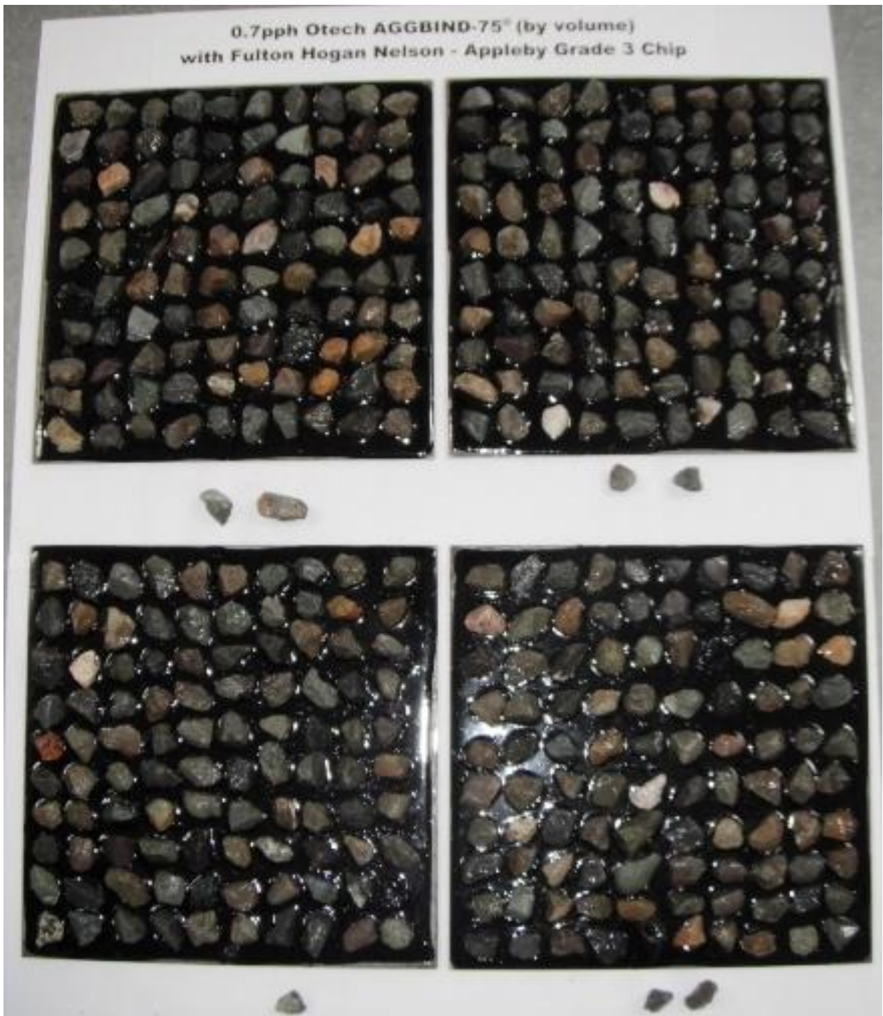
Figure 1. Photograph showing test plates with 180/200 bitumen and 0.7pph Otech AGGBIND-75® (by volume) after test was performed. Appleby grade 3 chip that was dislodged is arranged below the plates.
