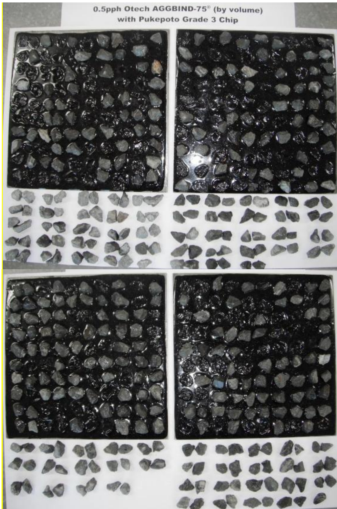
Figure 1. Photograph showing test plates with 180/200 bitumen and 0.5pph Otech AGGBIND-75® (by volume) after test was performed. Pukepoto Quarry grade 3 chip that was dislodged is arranged below the plates.
