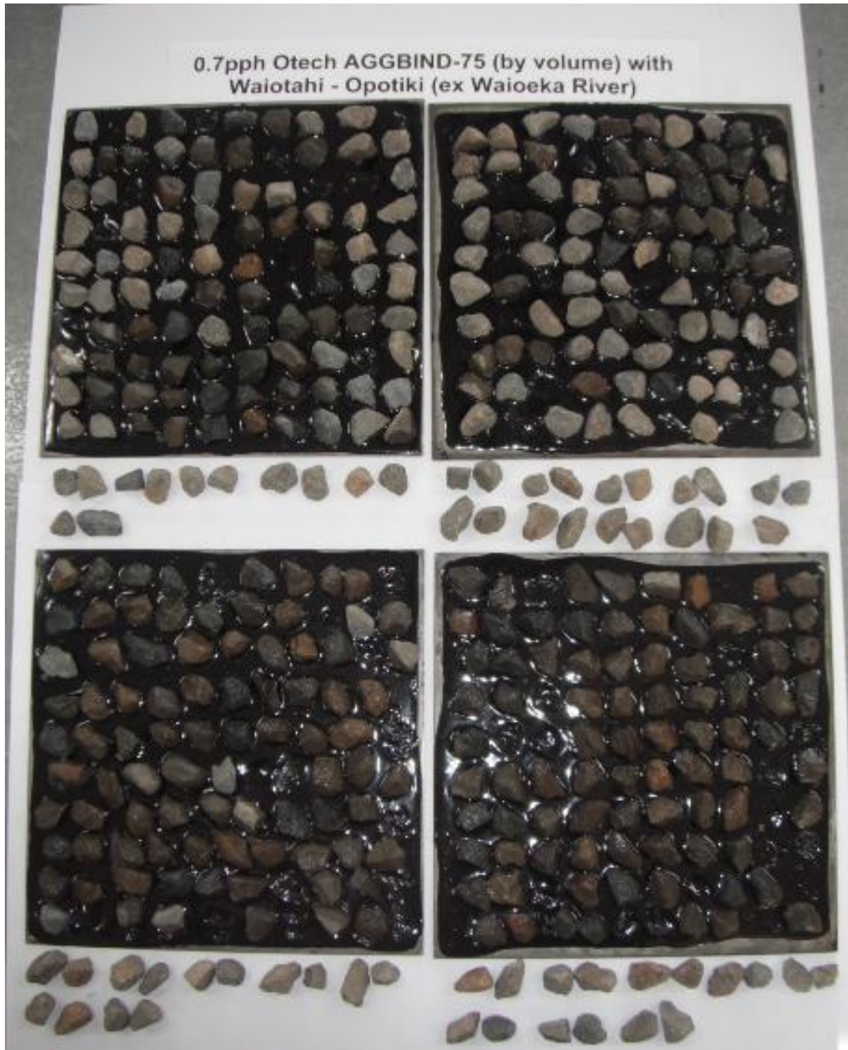
Figure 1. Photograph showing test plates with 180/200 bitumen and 0.7pph Otech AGGBIND-75 ® (by volume) after test was performed. Grade 3 Waiotahi – Opotiki (ex Waioeka River) chip that was dislodged is arranged below the plates.
