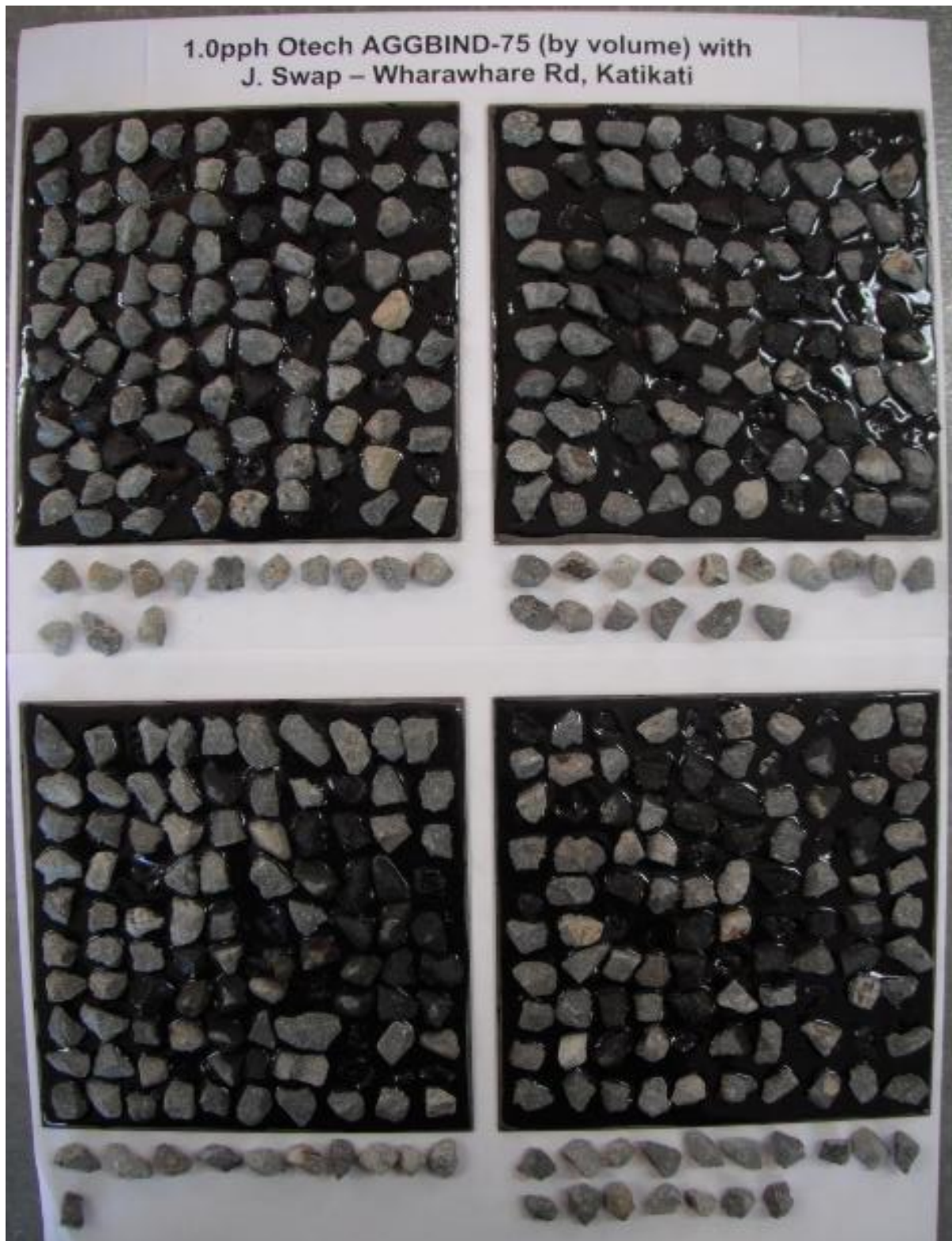
Figure 1. Photograph showing test plates with 180/200 bitumen and 1.0pph Otech AGGBIND-75 ® (by volume) after test was performed. Grade 3 Swaps – Wharawhare Road, Katikati chip that was dislodged is arranged below the plates.
