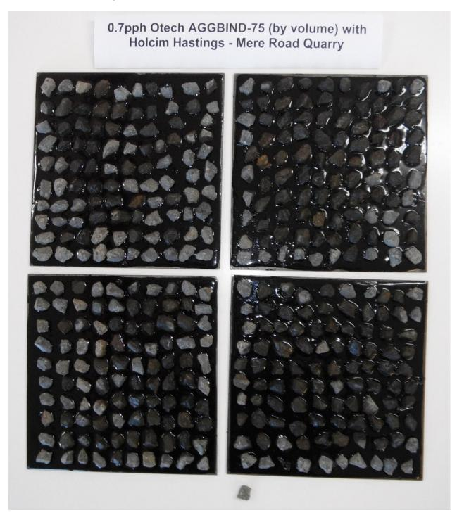
**Figure 1.** Photograph showing test plates with 180/200 bitumen and 0.7pph Otech AGGBIND-75<sup>®</sup> (by volume) after test was performed. Holcim Hastings - Mere Road Quarry Grade 3 chip that was dislodged is arranged below the plates.
