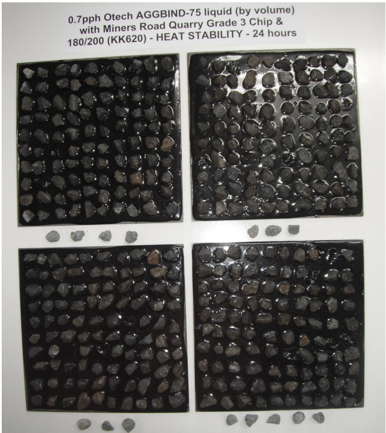
Figure 1. Photograph showing test plates with 180/200 bitumen and 0.7pph Otech AGGBIND-75 ® (by volume) after test was performed. Fulton Hogan - Miners Road Grade 3 chip dislodged is arranged below the plates.
