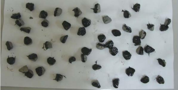
0.7% Otech Aggbind 75 Aggregate Condition: "SATURATED SURFACE DRY" Not Stripped (more than <sup>3</sup>/<sub>4</sub> of the contact area is coated with binder)
